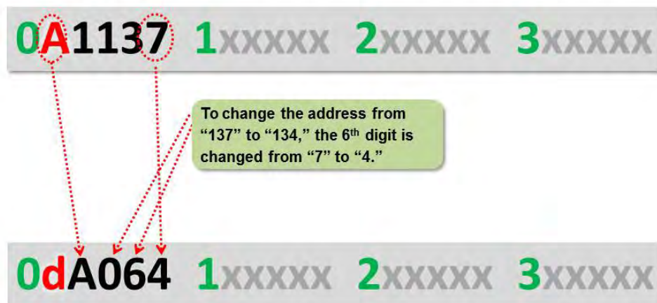
Figure 11. Example of using the specific digit changing mode to change a unit address
